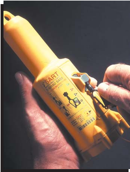
SARTs—Search and Rescue Transponders—direct rescuers to a target by emitting signals that are displayed on the rescue boat's radar.
